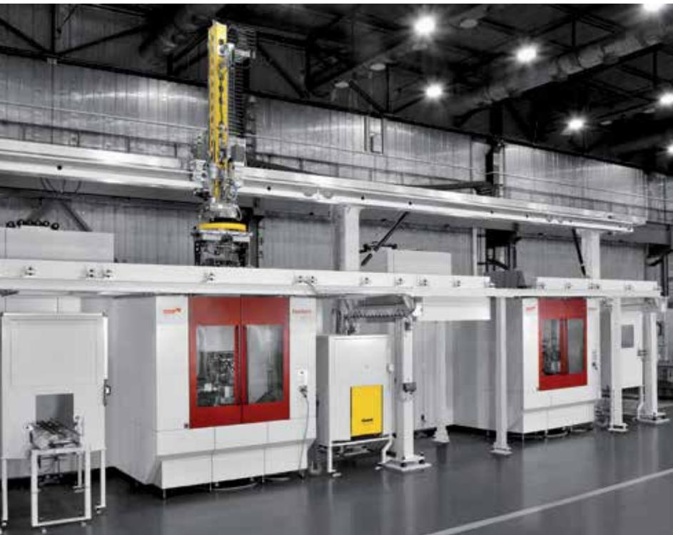
The machining centers HEC 500 / 630 / 800 Athletic have interfaces for the automatic workpiece, tool and information flow as a precondition for the integration into flexible production systems and production lines.
