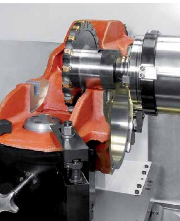
Ready-for-assembly complete machining of bush housings for the railway technology on the HEC 630 Athletic. Implementation as turn-key project from engineering to training and production support.
