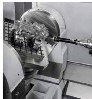
For a further reduction of the production time per work piece, increase of the machining accuracy and assembly-oriented production, the machining centers HEC 500 X5 / HEC 630 X5 / HEC 800 X5 are equipped with a combined NC rotary and pivoting unit. The advantages are the complete production in one clamping and the machining of slanting surfaces and holes without axis interpolation.
