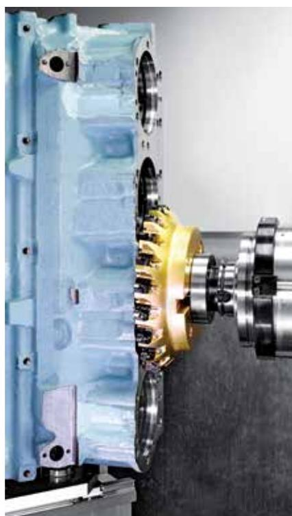
Semi-finish and finish machining of crankcases for V8 cylinder diesel engines in 2 clamping positions on the HEC 800 Athletic. High flexibility of machining different crankcases with universal clamping technology and the same tool sets.
