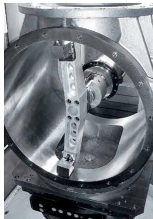
Production of housings for rotary feeders for bulk material dosage on the HEC 630 Athletic. Finish machining of the rotor bore hole up to a diameter of 120 mm with bridge tool. Production time reduction by 30 % as a result of fully automatic machining.
