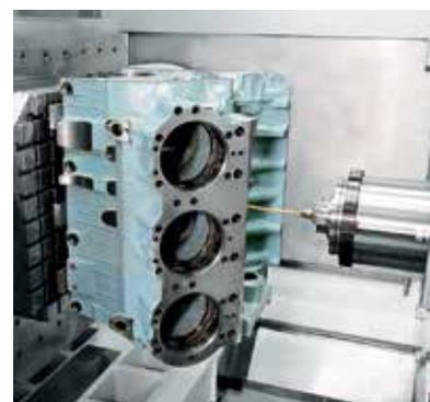
NC rotary and pivoting unit and tool tower magazine as option.
