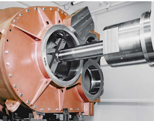
NC quill with stepless adjustment up to 500 mm or 760 mm.
